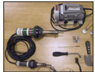
Figure 4 Standard tools needed for Heat Welding.
