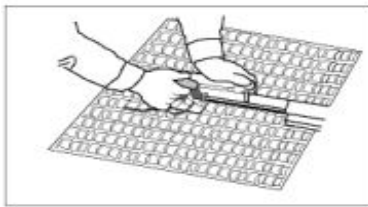
1. Groove the Seam
